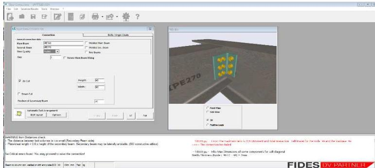
By double clicking a connection in the tree, the user can edit all the geometrical details, and see an interactive 2d or 3d view of the connection, as before. The loadcase editor can be invoked by each input form.
